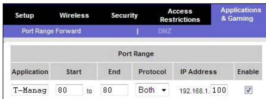
Forwarding port 80 on a Linksys router
